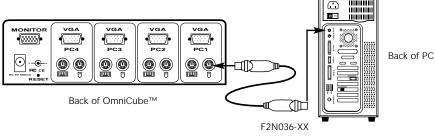
6. Connect the first computer's keyboard cable to the OmniCube<sup>™</sup>. Using another PS/2 cable (Belkin Part# F2N036-XX), connect one end to the PS/2 keyboard port on the computer, and the other end to the PC1 keyboard port on the back of the OmniCube<sup>™</sup>. If your computer has an AT-style keyboard port, you will need a PS/2-AT keyboard adapter (Belkin Part# F2N018).
